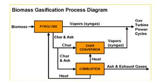
Another advantage of gasification is that it produces a fuel that has had many impurities removed and could therefore cause fewer pollution problems when burnt. Under suitable circumstances, it can also produce synthesis gas, a mixture of carbon monoxide and hydrogen which can be used to
